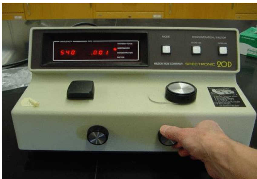
Figure 2: A single wavelength spectrophotometer.
